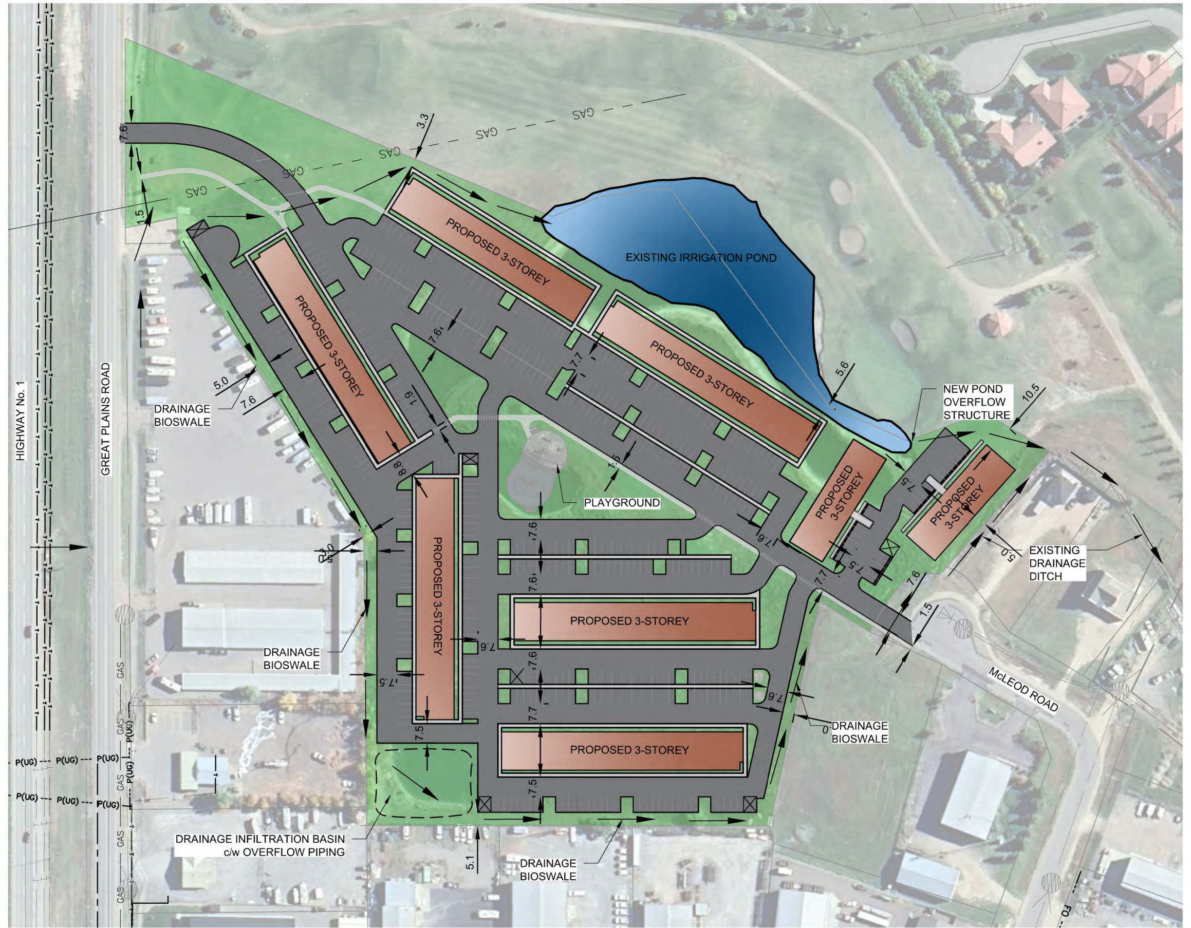
1 DRAINAGE CONCEPT PLAN SK-3 | 1:1500
