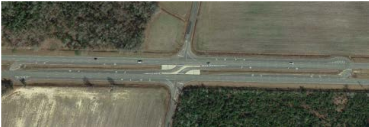
FIGURE 10: EXAMPLE RCUT INTERSECTION CONFIGURATION
