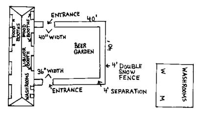
Dimensions are required for all areas to be permitted (label washrooms, bar area, kitchen, etc.); also show the width of entries/exits. Indicate type of enclosure for outdoor areas (must be 5' high or doubled with 4' dead space).
